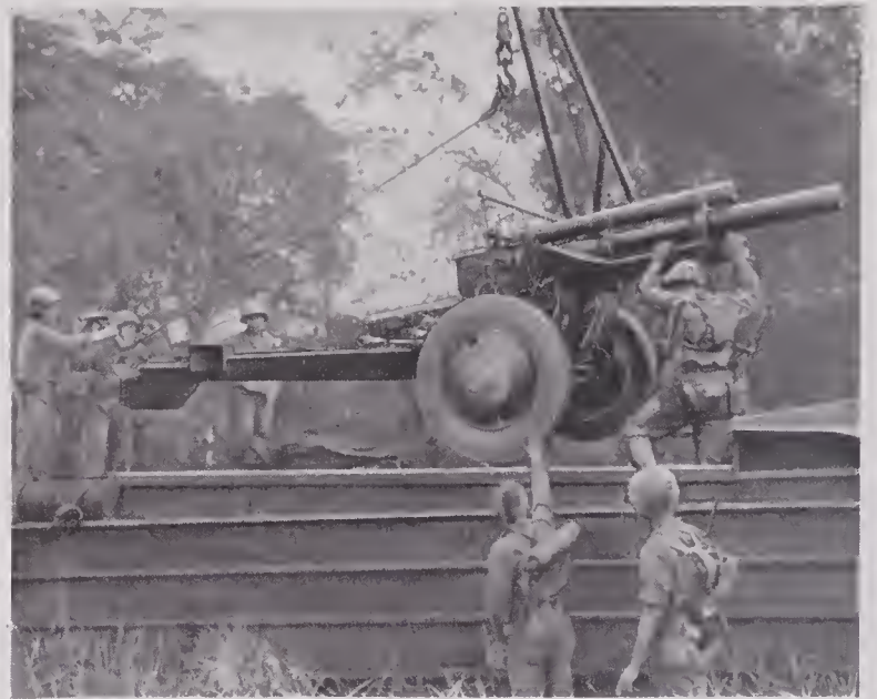
FIGURE 14. In OSRD-initiated demonstration, Milne Bay, New Guinea, 105-mm howitzer is lowered to ground after being lifted from another DUKW which has moved away and is waiting to tow piece into battery position.
